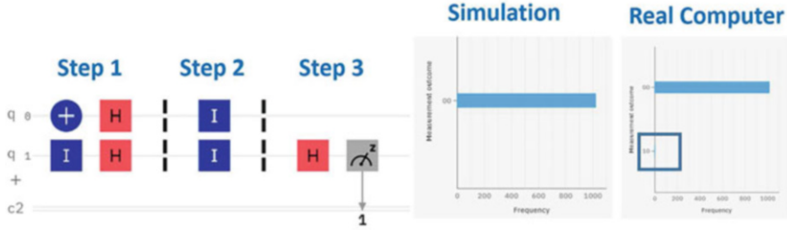
Fig. 21.3 Deutsch algorithm implemented in IBM-Q with a constant quantum oracle f(x) = 0 . Simulation and hardware results are shown on the right. MSB is at the bottom
