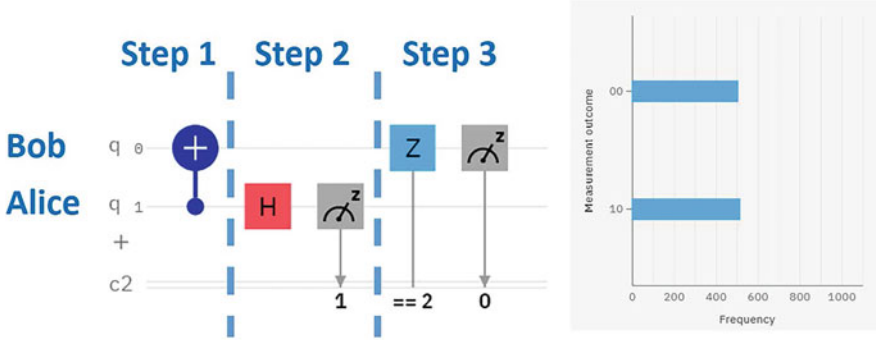
Fig. 19.2 Quantum teleportation circuit corresponds to Fig. 19.1 with |\Psi\rangle = |0\rangle
