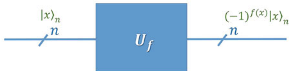
Fig. 22.2 A general phase quantum oracle. Note that |x\rangle_n is a basis vector
